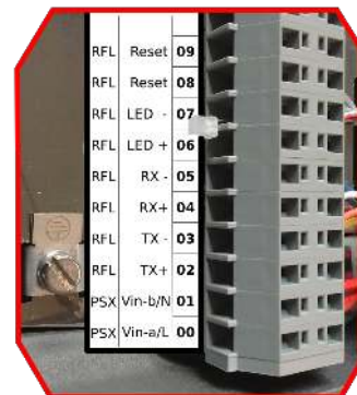
Figure 2.10: Terminal compartment and connections.
